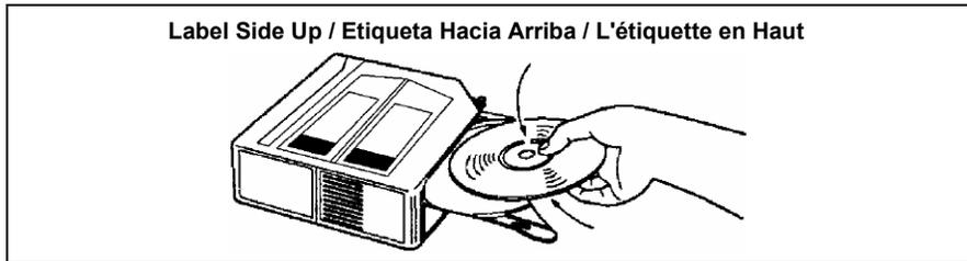
3. Push the tray back into the magazine. Load discs into the remaining 9 trays in a similar manner.
